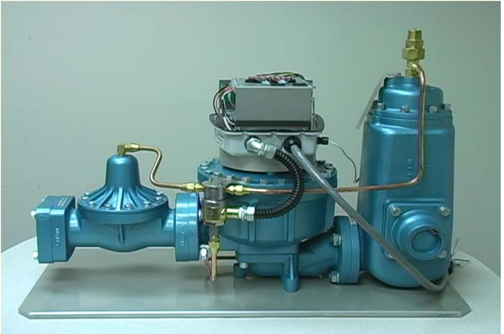
LPG Security Valve Installed on Meter
