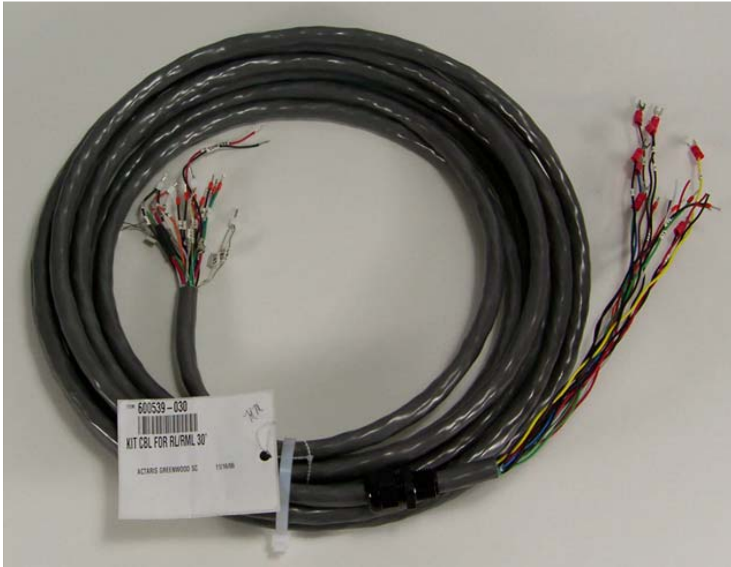
Prepped Power/Data Cable
